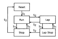
Starts functioning on the rising edge of S<sub>1</sub> and S<sub>2</sub>
