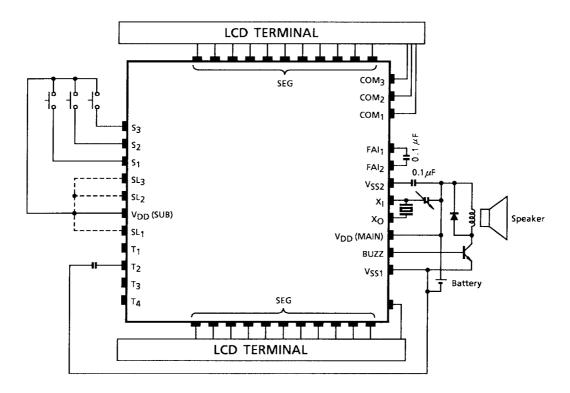
Note 11: Be sure to connect the  $V_{DD}$  (MAIN).
